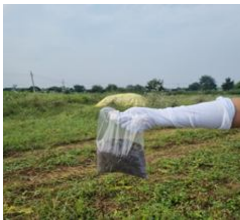
Fig. 6: On site soil sample packing.
